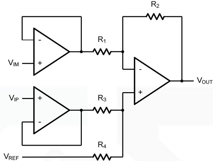
Figure 6. Instrument Amplifier
